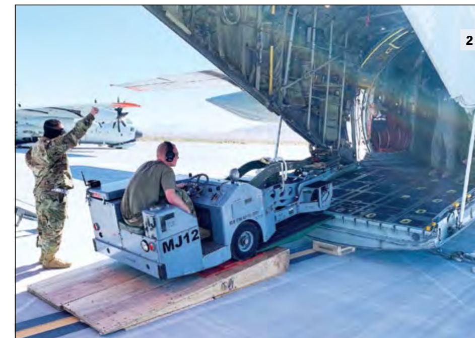
2) U.S. Air Force Airmen prepare to offload a weapon-loading jammer from a 109th Airlift Wing LC-130 Hercules aircraft Sept. 3 at Nellis Air Force Base, Nevada. Airmen are offloading cargo from the C-130 to prepare for an Integrated Combat Turn, which is the rapid re-arming and refueling of an aircraft.
